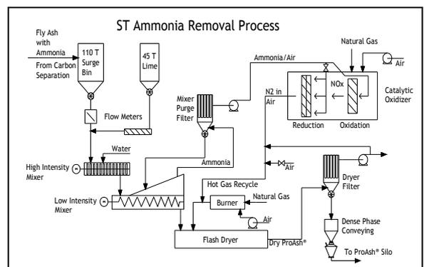
Fig. 3: STET Ammonia Removal System
