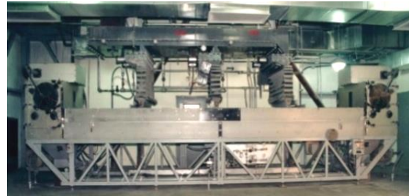
Figure 3. Commercial tribo-electrostatic belt separator.
